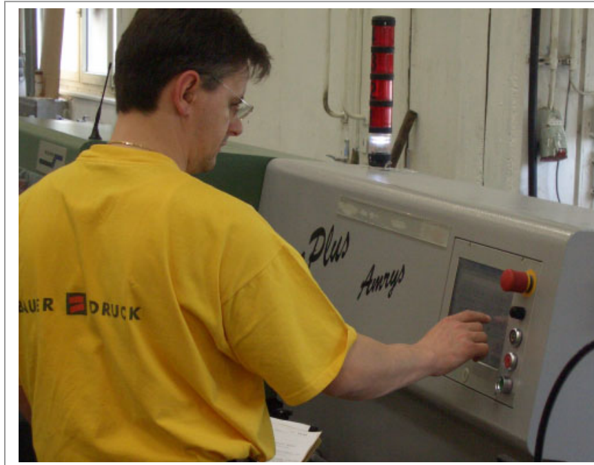
Photo 2: The Muller Martini AMRYS PrimaPlus saddle stitcher receives relevant job data from the Hiflex MIS.
